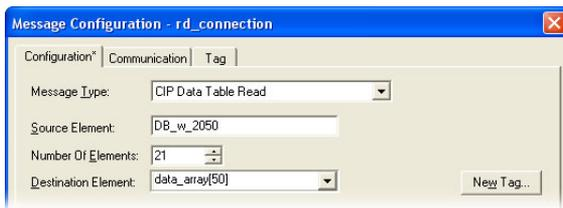
**Figure 67: MSG Instruction Configuration**
